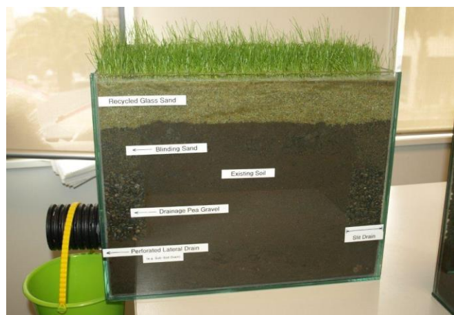
Figure 12: Photo showing proposed ryegrass, glass sand layer, and drainage options for Trafalgar Park
